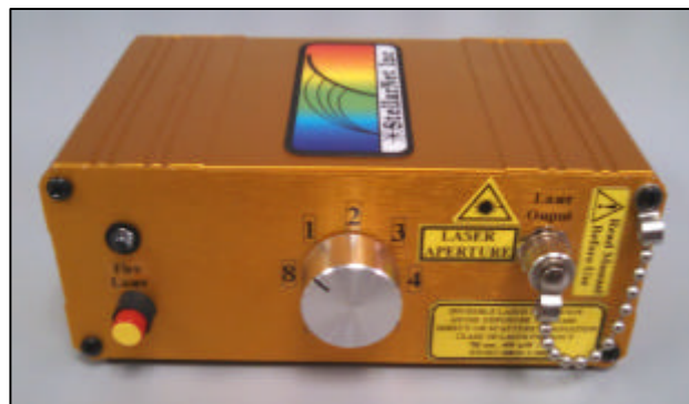
RamuLaser accessory attaches to Raman probe
