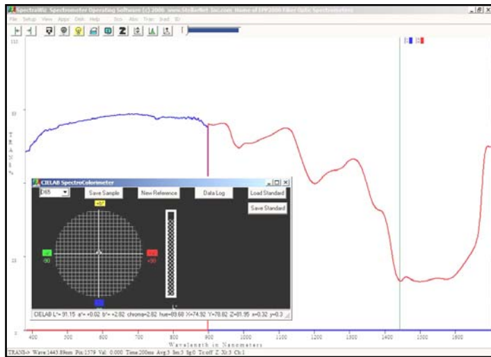
Dual-DSR reflectance spectrum of white sugar showing color and CH composition using TXF1 reflectance fixture for 280-1700nm
