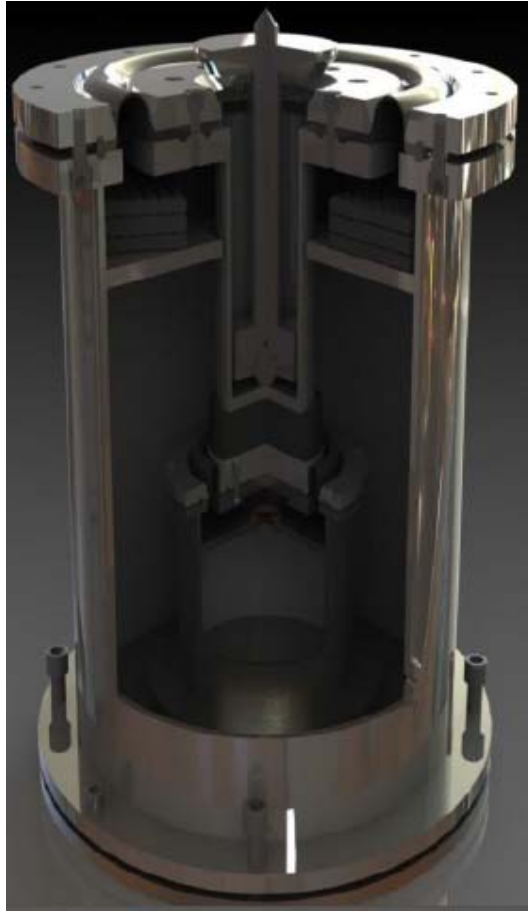
Bulb Self-centering Pendulum-bar Isolator with Air Chambers
